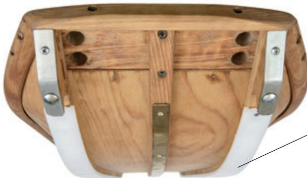
REPLACEABLE GLIDING SYSTEM. All sledges can be equipped with our new replaceable gliding system. It consists of a bottom strip in aluminum on which a plastic runner is attached. The plastic runner can easily be replaced when worn out. 'This kind of system is used by sledge dog drivers across the world. You can also get your sledge with brass strips on the runners. It will not glide just as well as the plastic runner but are extremely durable.
