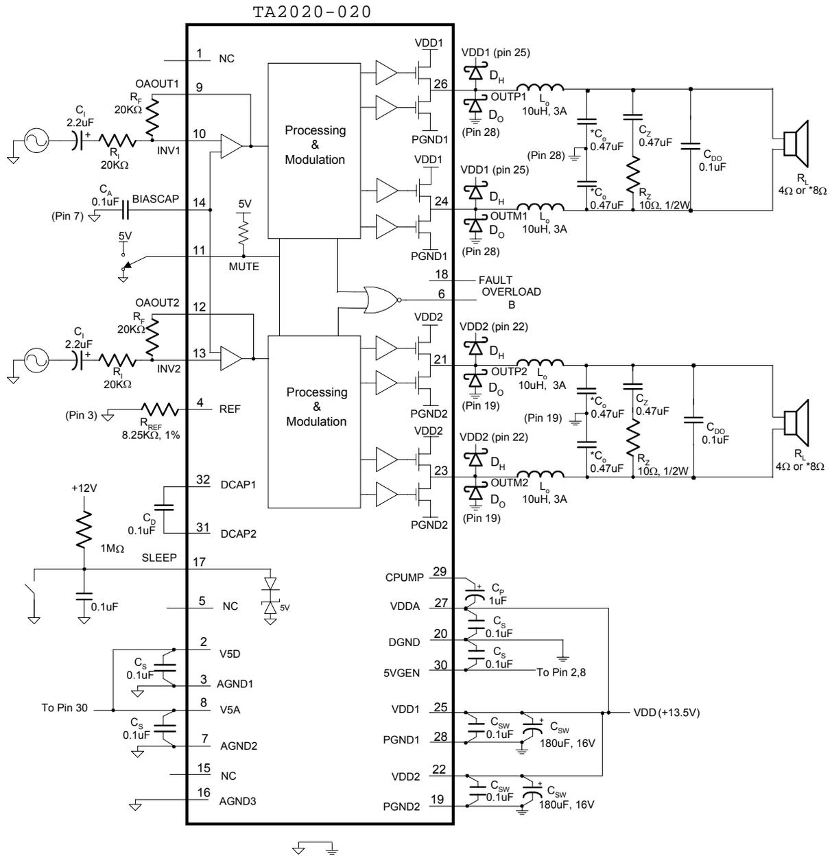
Note: Analog and Digital/Power Grounds must be connected locally at the TA2020-020
