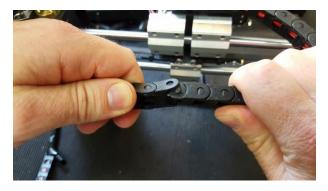
2. Push about 2 cm of cable into the drag chain so the crimp will end up outside the chain closest to the extruder.
