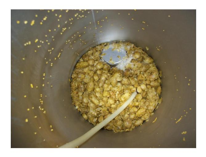
FOR THE PURIST OUT THERE, HERE IS A KEG THAT WAS DRY HOPPED WITH 1  $\frac{3}{4}$  OZ OF WHOLE HOPS. HOW THE SYSTEM ORIENTATES ITSELF IS NOT AS PREDICTABLE AS WITH PELLET HOPS, BUT IT WORKS FINE AND AGAIN, CLEAR, CLEAN BEER UNTIL THE END.
