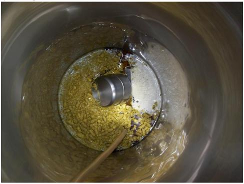
THE KEG IS BEING FILLED STRAIGHT FROM THE FERMENTER THROUGH THE "OUT" PORT. USE THE KEG AS THE SECONDARY FERMENTER, THERE ARE SO MANY ADVANTAGES TOO NUMEROUS TO LIST HERE. YOU CAN RACK STRAIGHT INTO TO THE KEG VIA OTHER MEANS IF DESIRED. (NEXT PAGE)
