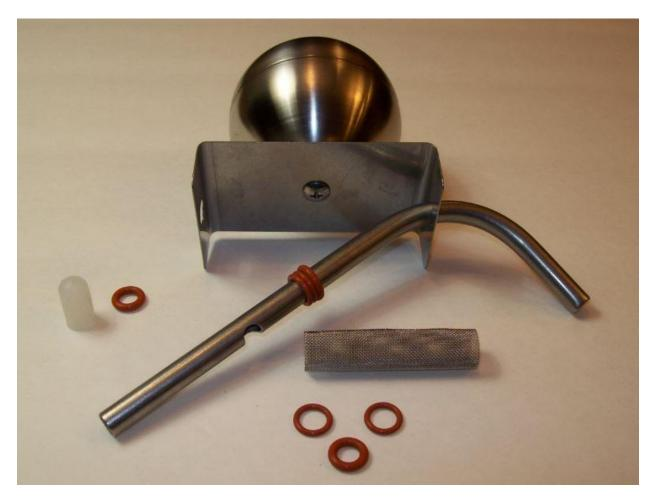
ROLL ONE LARGE DIAMETER O RING FOLLOWED BY TWO SMALL DIAMETER O RINGS ONTO THE STRAIGHT SECTION OF TUBE AND POSITION THEM ABOUT 1" FROM CENTER OF INTAKE PORT. BE CAREFUL WHEN ROLLING THE O RINGS OVER THE INTAKE PORT. DO NOT USE EXCESSIVE FORCE OR YOU COULD CUT THE O RINGS. HAVING THEM WET WITH STAR SAN WILL HELP WITH THIS PROCESS.
