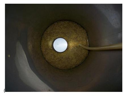
PARTICLE FREE, CRYSTAL CLEAR BEER WAS DISPENSED UNTIL THE END. NO CLOGGED POPPETS, TUBES, OR HOSES. FANTASTIC HOP AROMA AND FLAVOR! ONCE THE INTAKE PORT IS SUBMERGED IN THE HOPS, OR SITTING RIGHT ON TOP OF THE HOPS, THE BEER WILL START TO POUR FOAMY, WHICH OBVIOUSLY MEANS THE KEG IS ABOUT GONE. IF YOUR DESPERATE FOR 1 LAST PINT, LET THE KEG SIT FOR A DAY OR TWO, YOU MAY GET ONE MORE TASTE OF HOPPY GOODNESS! (NEXT PAGE)
