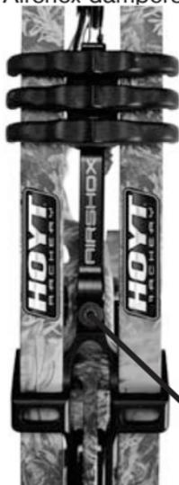
Always remove the AirShox extension arms while pressing the bow in a bow press or when disassembling the bow, failure to do so may cause damage to the bow. Damage to the bow as a result of not removing the AirShox extension arms for bow press usage is not covered by warranty. Remove the extension arm by removing the set screw. Re-install after all adjustments are completed and do not over-tighten the set screw.
