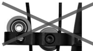
When installed correctly the cables will not touch each other. (See figs. 4 and 5). It is not necessary to remove the roller wheels to change the buss and control cables on 2013 models.
