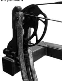
Proper representation of how limbs should be pressed
