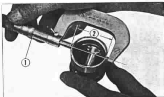
① Micrometer ② Piston diameter Fig. 30
