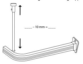
6. Cut the ceiling support pipe into suitable length.
