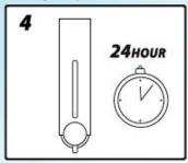
Hold in place for one minute. Do not fill container for 24 hours to allow the silicone time to fully dry.
