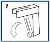
Open the back of the unit. Press on the button and pull on the front panel. Remove the refill container.
