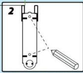
Put the unit in place. Hold the back plate against the wall and mark the location of the screw holes.
