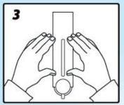
Make wavy lines of silicone on back of the dispenser where it will touch the wall. Please use all of the tube for maximum bond. Press firmly onto wall.
