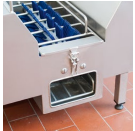
Separate cleaning of sole and upper shoe
