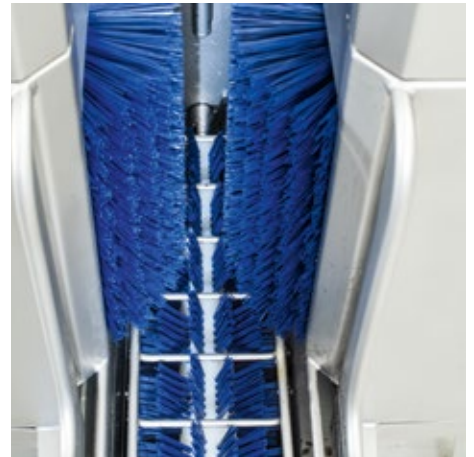
Roller brushes made from nylon
