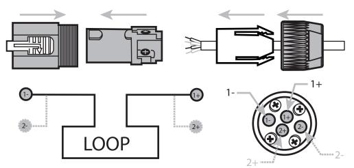
1 = Twisted Pair positive & negative , 1 & 2 = Quad Core positive and negative connections.
